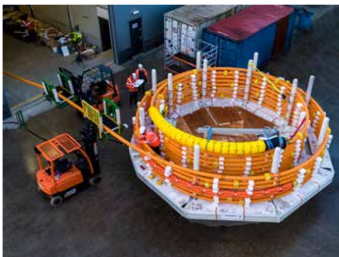
TCP can be delivered on subsea pallets and installed using smaller vessels
