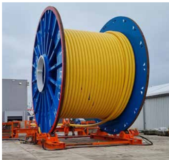
TCP is flexible and can be delivered in long lengths on reels
